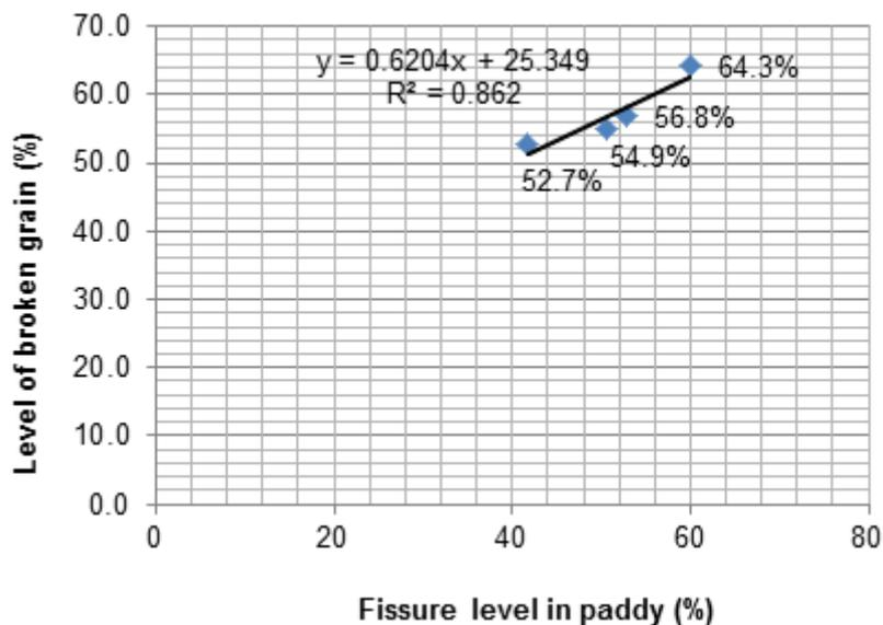
Figure 3. Correlation of levels of fissure in paddy and broken grain in milled rice.
